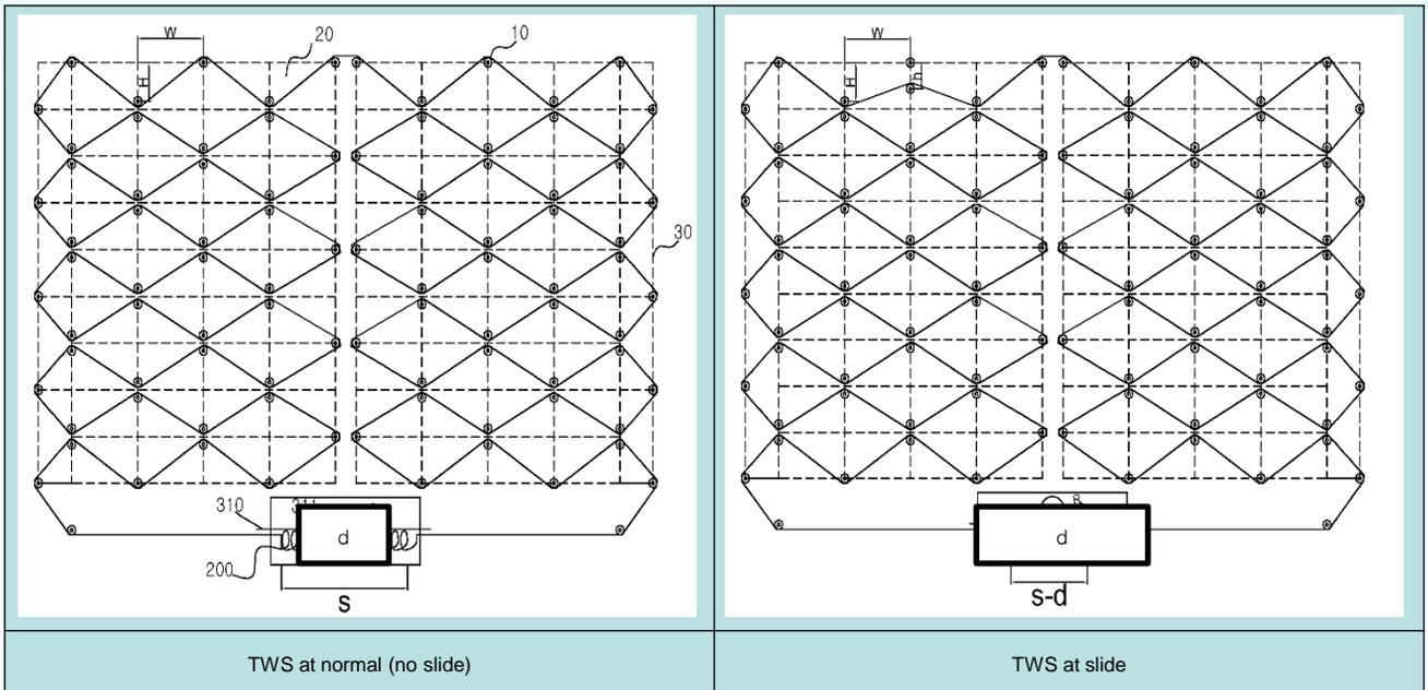
The entire surface vulnerable to slide or fall shall be covered with **TWS** (Tension Wire Screen) which is composed of a tiny stainless wire ( typically 1.2mm diameter) in Zig-Zag pattern under tension. Any slide or fall shall disturb the initial TWS pattern so as to activate the **FODS** (FO Displacement Sensor) positioned on the bottom TWS and trigger alarm at exceeding the predetermined limit value.
