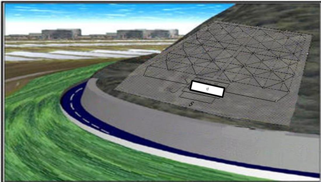
Cover a soft surface vulnerable to slide or fall with TWS and connect it via FOC to the remote OMU.
